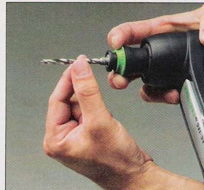
The C12 ships with a hex drive chuck. It's ideal for switching out bits quickly.
