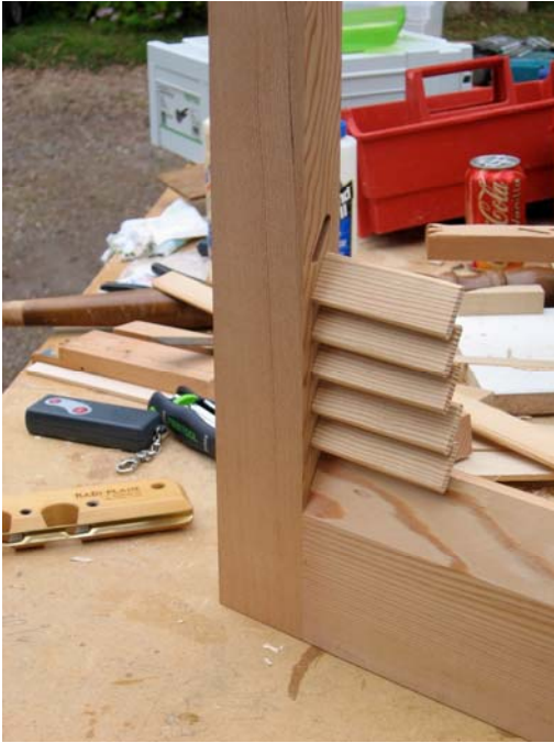
Photo #1: As you can see, beveling the rail to match the louver angle exposed too much flat-sawn grain on a quarter-sawn project.
